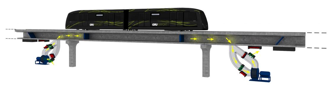
The system uses pneumatic energy for propulsion generated by stationary centrifugal blowers that feed and/or evacuate air from a duct. The vehicles travel guided by conventional running rails. Acceleration is determined by the combination of pressure and airflow within the propulsion duct, controlled by adjusting the blower rotation speed and positioning valves.
