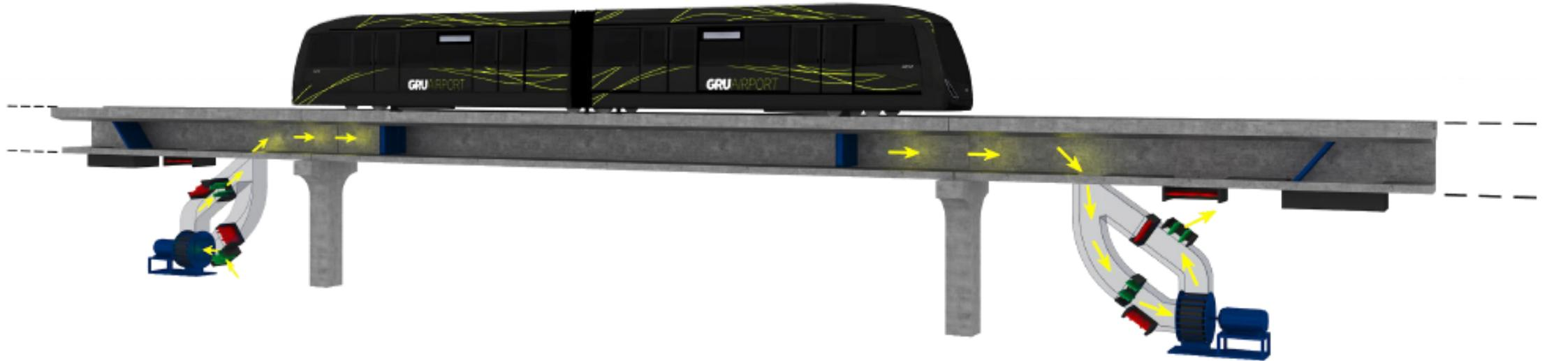
The system uses pneumatic energy for propulsion generated by stationary centrifugal blowers that feed and/or evacuate air from a duct. The vehicles travel guided by conventional running rails. Acceleration is determined by the combination of pressure and airflow within the propulsion duct, controlled by adjusting the blower rotation speed and positioning valves.
