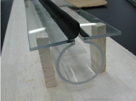
Fig.3 Photo showing acrylic plates and rubber sheets on the top of acrylic pipe
