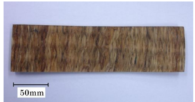
Fig.5 A kenaf blade fabricated by a hot press
