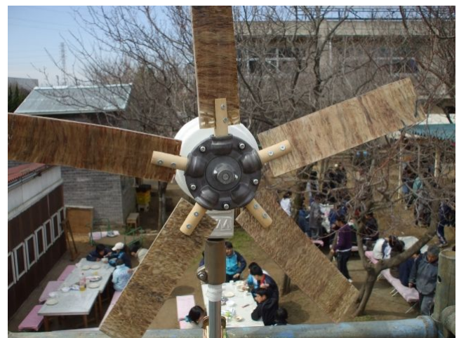
Fig.6 Biodegradable blades, made by students and authors, fitted into a small wind turbine
